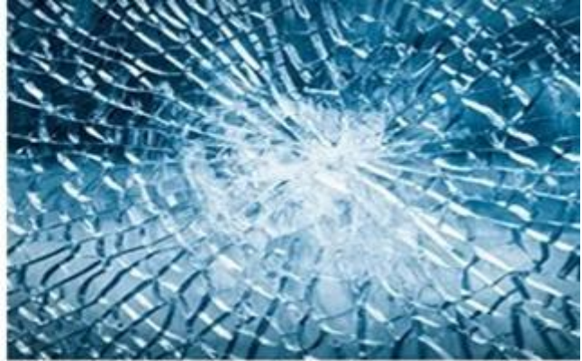
Tempered glass breaks into many small pieces with less sharp edges.
