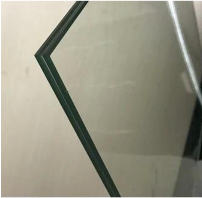
10.76 thick clear laminated glass application:
