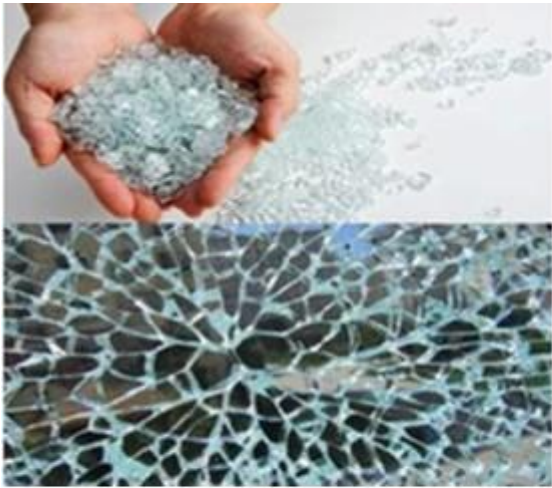
Toughened Glass broken into alveolate granules is human harmless
