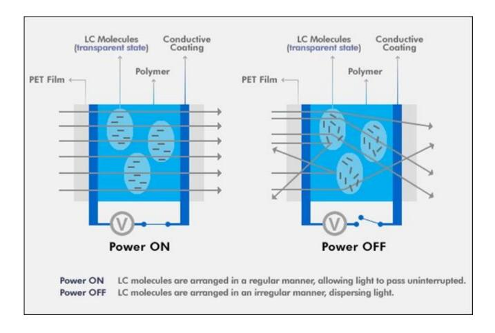
Electric privacy glass floor us on the walkways, when turn on the PDLC film, it become transparent and seem dangerous; when turn off, it's opal color and looks like the normal safety glass floor.
