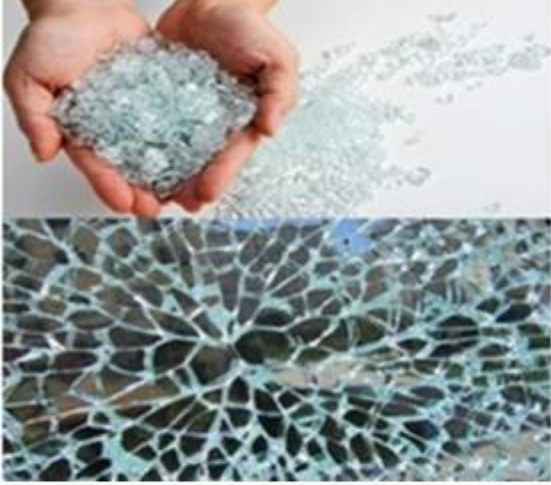
Toughened Glass broken into alveolate granules is human harmless
