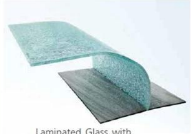
Laminated Glass with PVB Interlayer
