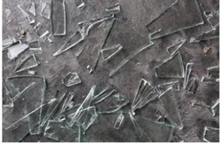
Annealed Glass when broken into sharp, easy to hurt human
