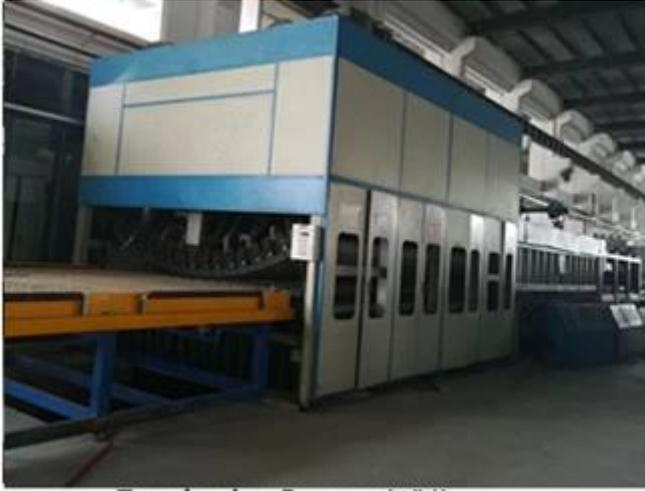
Toughening Furnace 钢化炉
