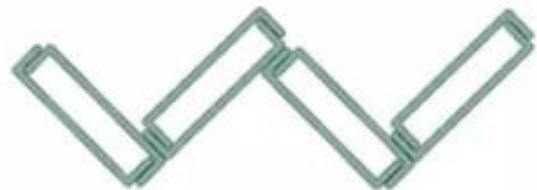
Double glazing arranged in zig-zag formation in pairs
