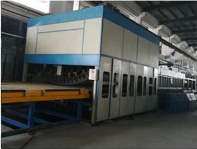
Toughening Furnace 钢化炉
