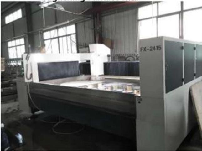
CNC edge grinding machine CNC磨边机
