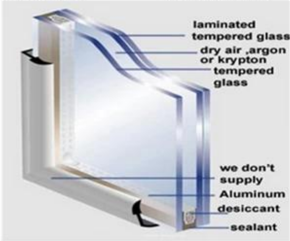
5. tempered & laminated insulated glass
