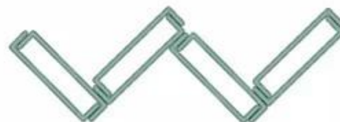
Double glazing arranged in zig-zag formation in pairs
