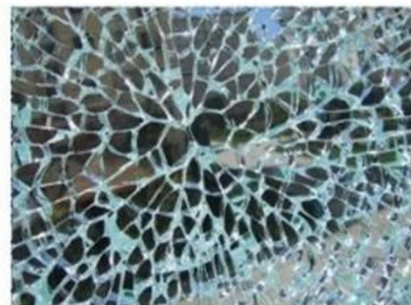
Tempered laminated glass with very strong external force cubical debris will fall down
