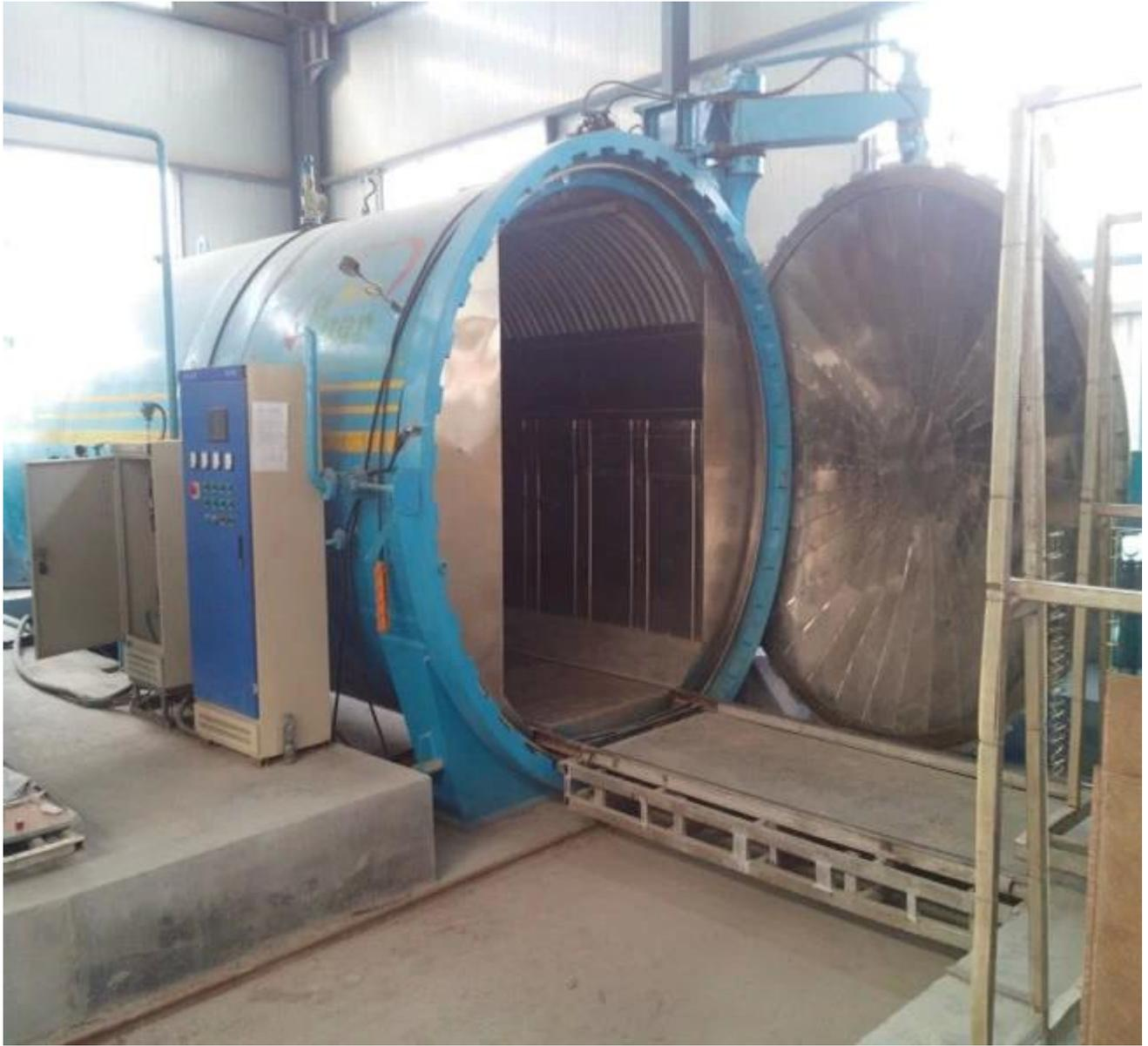
Figure 11.14: A large industrial autoclave used for sterilization of medical equipment.
