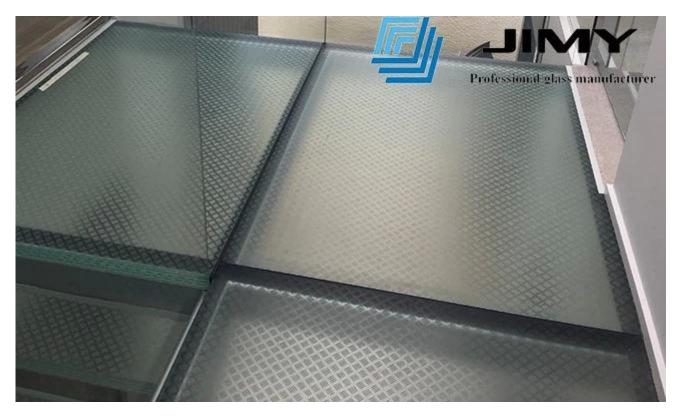
39.04mm anti-slip floor glass is make up of 3 layers of 12mm tempered glass permanently bonded together with 2 inter layers of 1.52mm PVB/SGP film via a controlled, highly pressurized and industrial heating process. The lamination process results in the glass panels holding together in the event of breakage, reducing the risk of harm.
