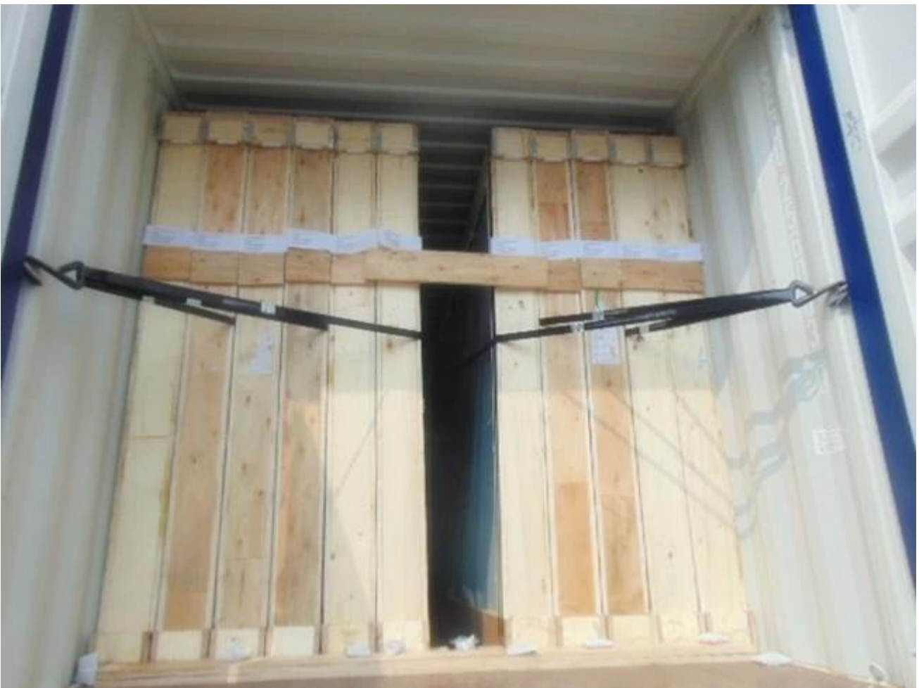
Glass Safety Loading
