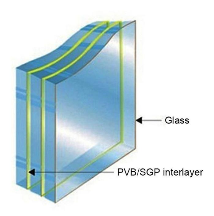
Annealed glass VS monolithic tempered glass VS laminted glass:
