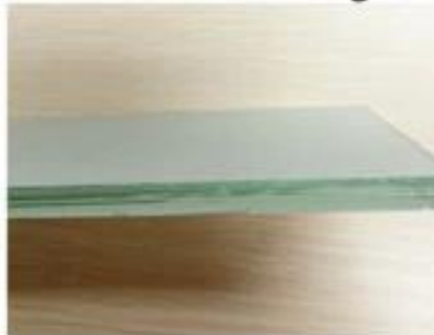
acid etched laminated glass
