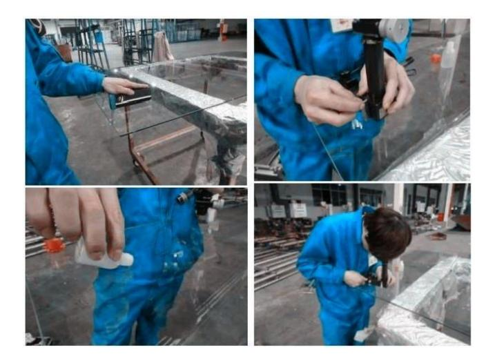
3.When laminated processing, make sure the temperature is 15-25 Celsius, humidity 20-28%, use ruler check the two layers of glass whether flush
