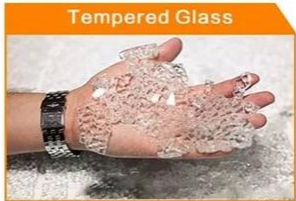
Qualifies as safety glazing
