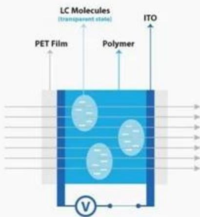
**Power ON** : By changing the orientation of the liquid crystal molecules with an electric field, it is possible to vary the intensity of transmitted light.
