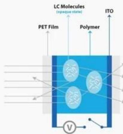
**Power OFF** : As liquid crystal molecules are randomly orientated, restricting lights from passing through.
