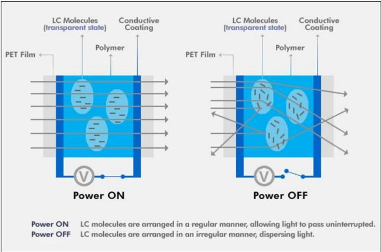
PDLC cell diagram showing the transition between transparent and opaque states based on the application of voltage.
