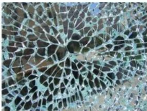
Tempered laminated glass with normal external force cubical debris won't fall down
