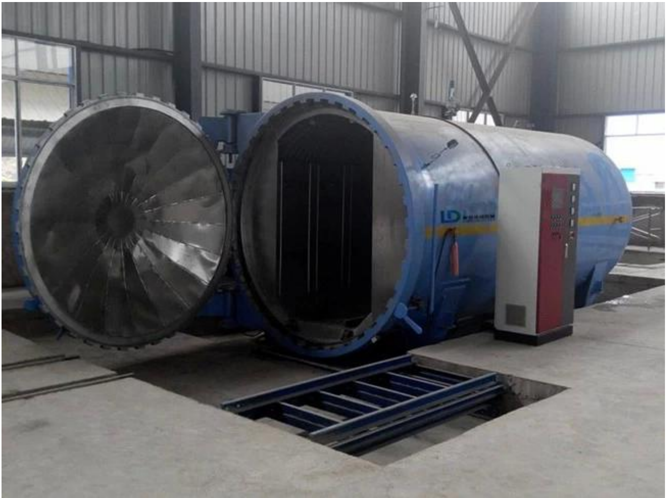
Laminated Glass Autoclave
