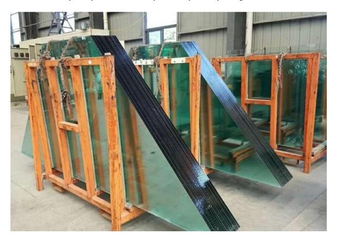
The finished glass product after boned of a layer of euro grey PVB/SGP film, it is special shaped tempered laminated glass panel show as below:
