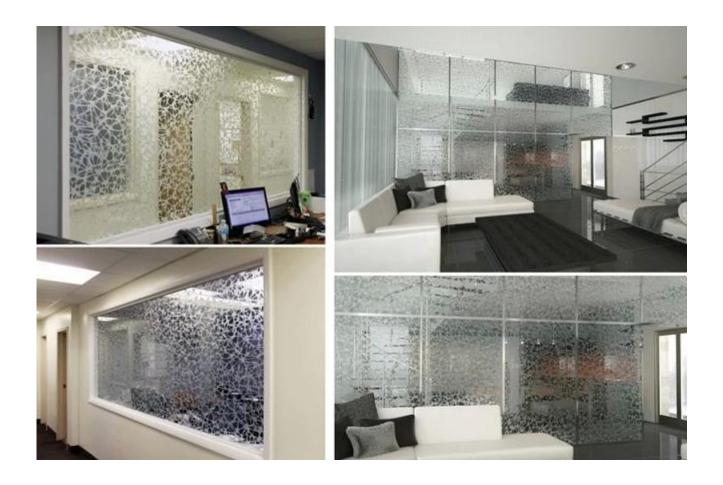
Other special design graphics acid etched glass apply for glass partition wall
