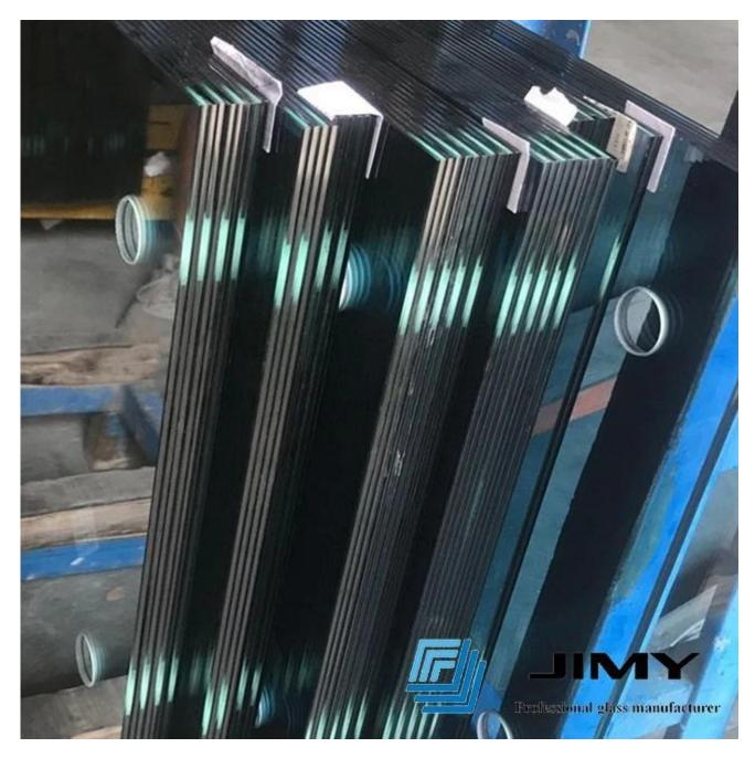
3.If hole drill is required, we suggest 1.14mm PVB at least; If groove cut or curved shape is required , we suggest 1.52mm PVB at least.
