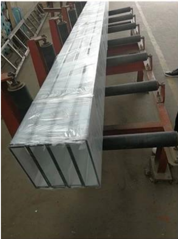
10mm low iron U profile glass application
