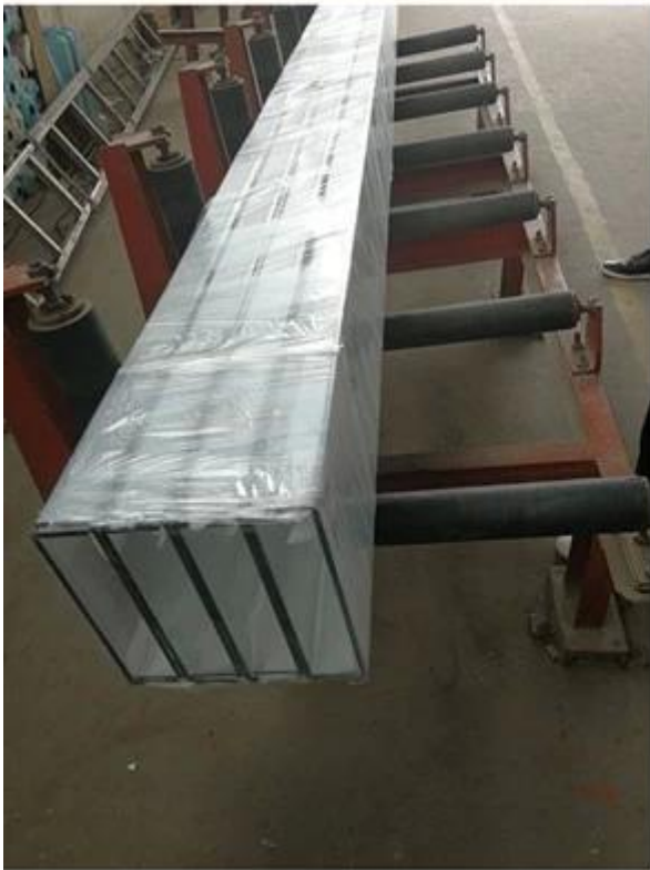
10mm low iron U profile glass application
