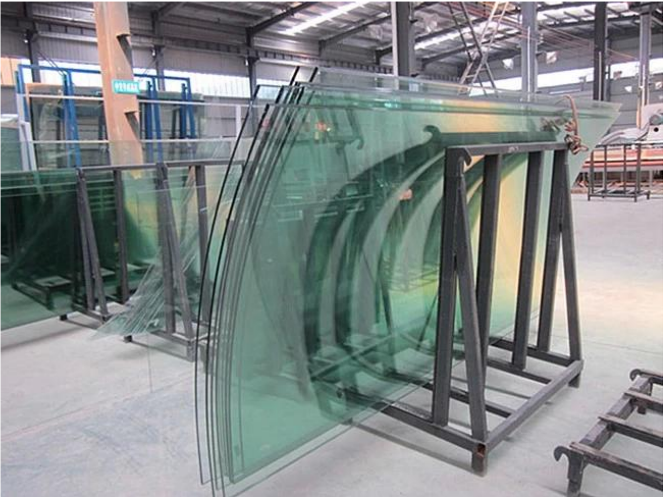
Arched tempered glass workshop
