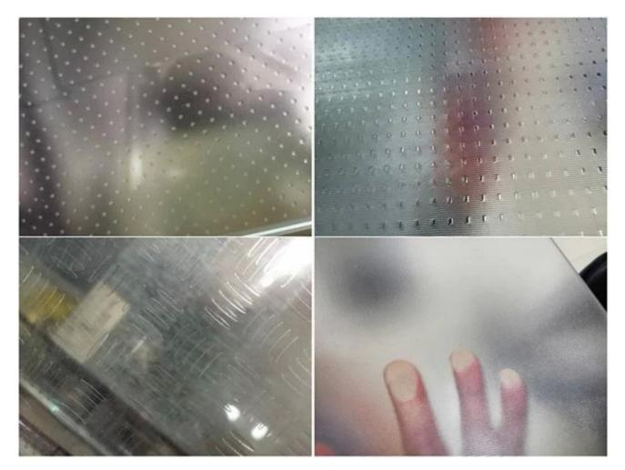
View of 48mm extra clear acid etched SGP laminated tempered glass floor panels
