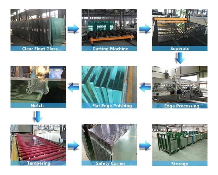
2. We have skillful workers to operate the machines and professional inspectors to inspect the glass piece by piece, to make sure the high quality of each glass panel, and our glass already tested and approved by CE EN12150 and SGCC Z97.1;
