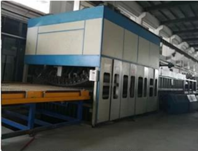
Toughening Furnace 钢化炉
