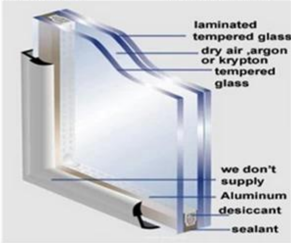
5. tempered & laminated insulated glass
