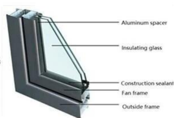
Aluminum spacer insulated glass
